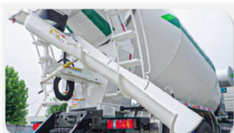
Extended discharge chute
